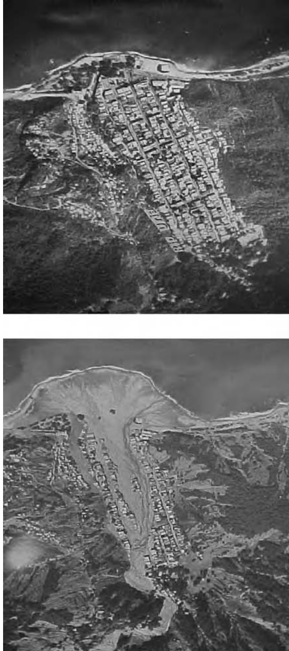
FIGURE 16.10 The plan for preventing future major mudslide events included the installation of slope and grade controls within upper reaches of the drainage ways, rock dams, and larger cement lined channels to convey materials to the ocean. (Such as those used in Caracas, Venezuela). This strategy has proven to be ineffective.
