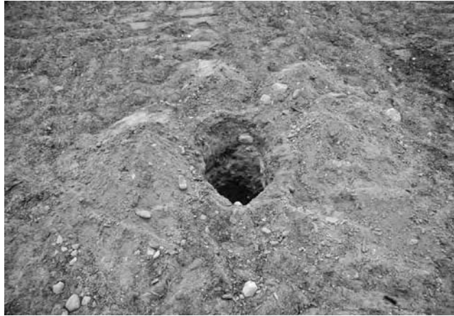
FIGURE 2.19 An auger hole through the topsoil and into the subsoil to examine apparent soil density, Spectacle Island.
