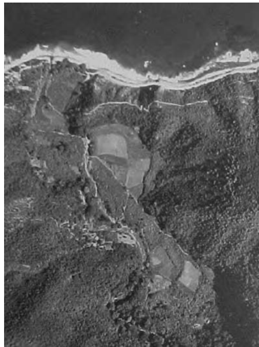
FIGURES 16.9 The predevelopment agricultural valley was eventually constructed. Cement lined channels that conveyed regular minor mudflows directly to the ocean became blocked by massive rocks and mud materials during the event. As a result, the mudflows diverted through the urban areas, destroying communities and killing thousands of people.
