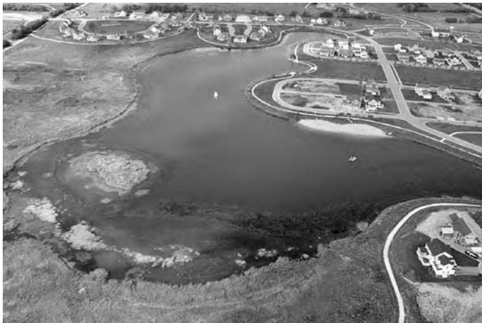
FIGURE 16.6 We use alternative stormwater management that requires a stormwater treatment train (STT) comprised of linked series landscape features that manage the volume, rate, and quality of stormwater simultaneously. We have used this strategy in projects and reduced total volume of runoff by over 50–75%, and reduced peak discharges by over 60%. This technique can eliminate storm sewers, save money, and greatly improve water quality in lakes (Apfelbaum 2004).
